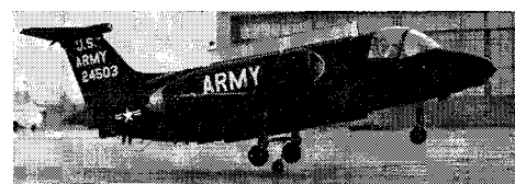
Fig. 21 Lockheed XV-4A (Hummingbird) turbojet-ejector V/STOL research airplane.
